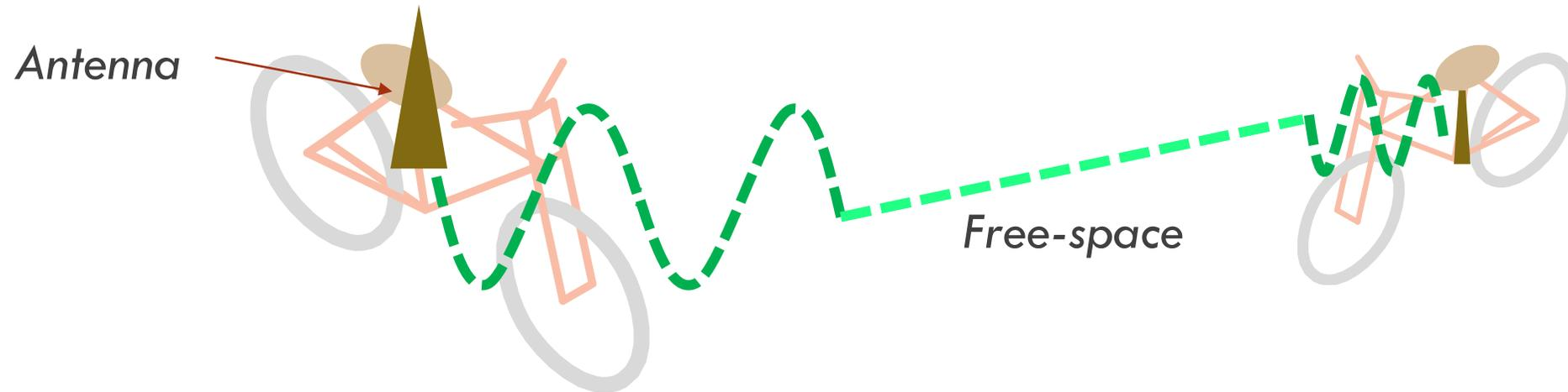
$$P_{rx} \text{ [dBm]} = P_{tx} + \underbrace{L_{\text{free-space}}(d)}_{\text{(e.g., Log-distance Path Loss)}} + G_{B-A(tx)}(p, \alpha) + G_{B-A(rx)}(p, \alpha)$$
