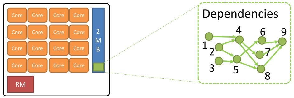
The essential openMP task dependency information is captured within a streamlined data structure hosted in the on-cluster shared memory
