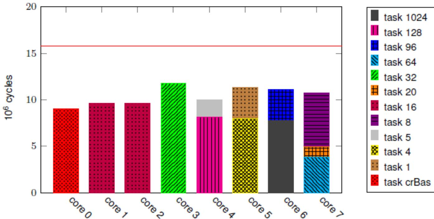
per core task allocation with combined parallelization approach
