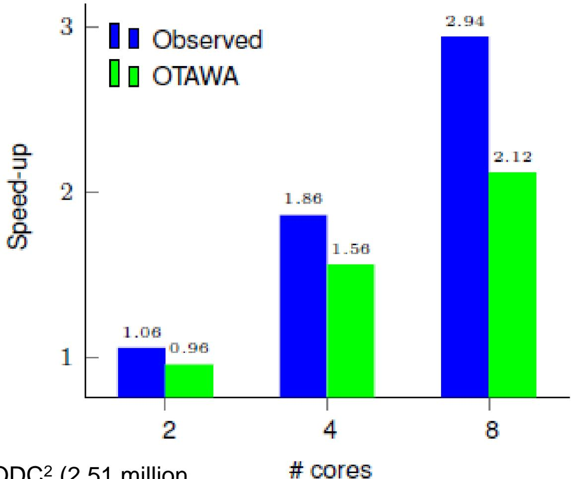
Observed execution time with ODC<sup>2</sup> (2.51 million cycles) is very close to a cache with perfect coherency protocol (2.42 million cycles for 8 cores)
