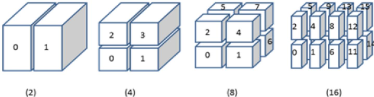
3D path planning: Laplacian multi-grid algorithm parallelised by obstacle map partitioning
