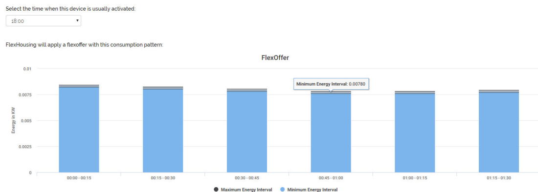
Fig. 31 – Automatically creating the consumption pattern for a Flex-Offfer in the new FlexHousing web platform.
