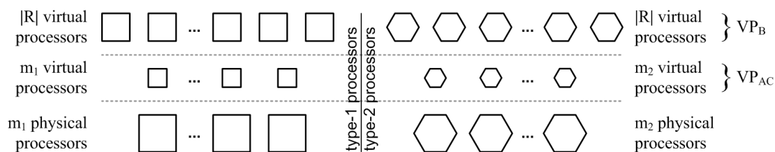
Figure 5.6: m + 2|R| virtual processors created from m physical processors on a two-type heterogeneous multiprocessor platform ( m = m_1 + m_2 ).
