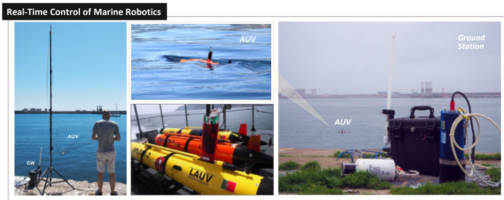
Figure 1.2: A set of illustrative examples of an AUV in real-world operation. It includes the so-called Manta gateway (GW) on the right and left pictures. The two middle image shows an AUV on the water (middle-top) and outside the water (middle-bottom) on a boat before a mission.
