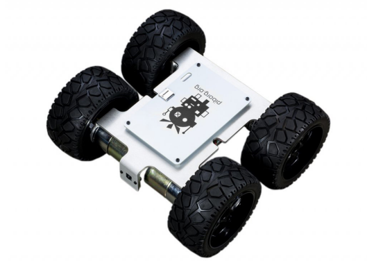
Figure 2.3: Monsterborg - The robotic platform used in the Formula Pi competition [3]
