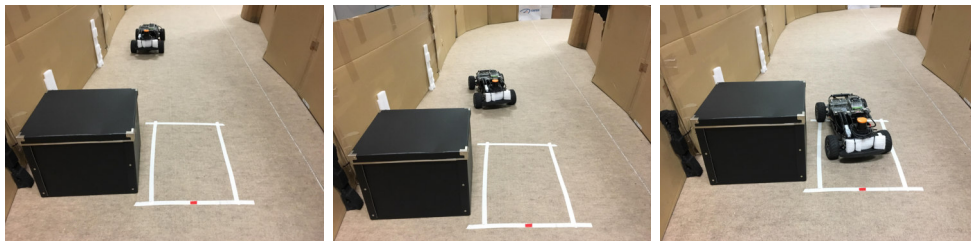
Figure 6.22: Demonstration of the racecar avoiding an obstacle in real life.
