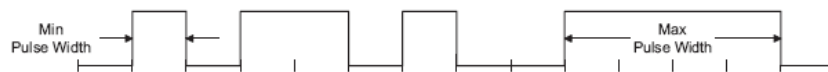
Figure 45 Minimum and maximum pulse width in a non return to zero (NRZ) bit encoding [52]
