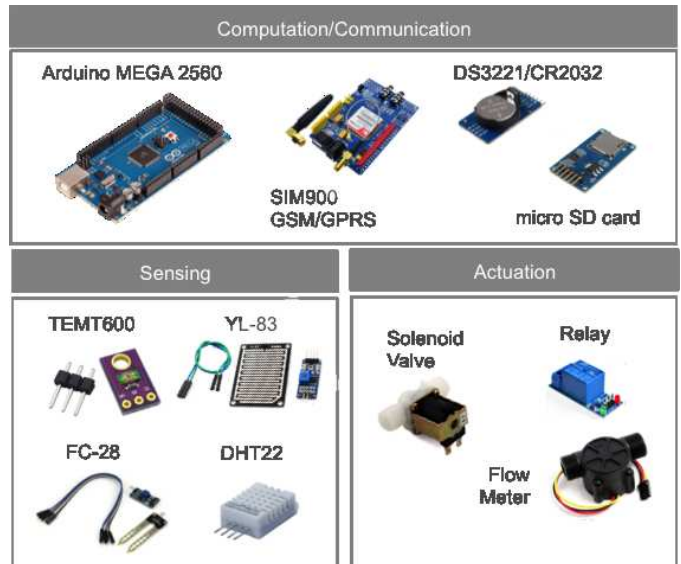
Fig. 2. A view of the main hardware used for the cropland station.
