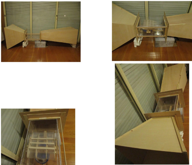
Fig. 25. Wind tunnel with open design according to the guidelines in [31].
