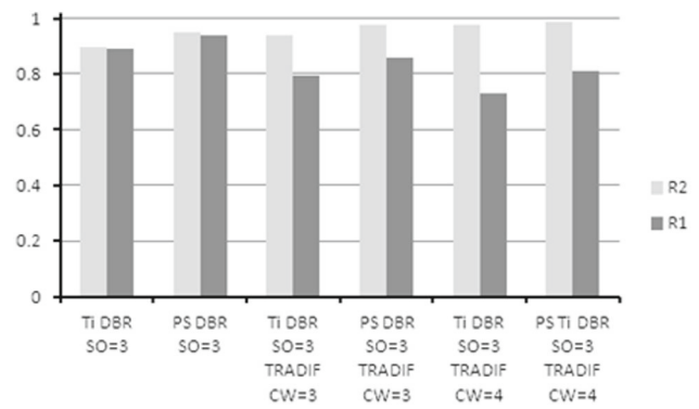
Fig. 12 Average probability of successful transmissions and average T_i for different contention windows at two routers
